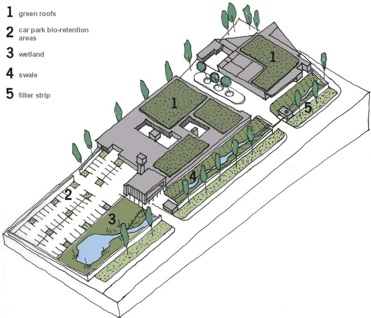
Figure 6.18 : Incorporating SuDS on industrial sites
